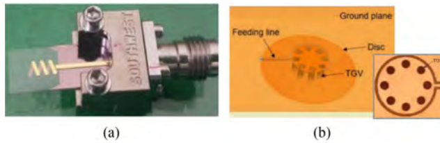
FIGURE 15. Antennas based on TGVs. (a) End-fire helix at 58 GHz [153] (b) AiP monopole at 62 GHz [154].
